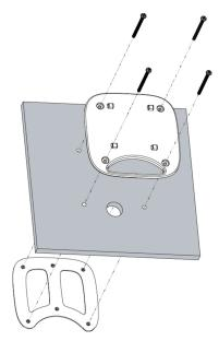
Push the provided drywall anchors into the drilled holes, then place the mounting bracket snugly against the wall. Using a screwdriver, screw the wall mount screws into the drywall anchors.
