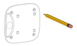
2. Attach the mounting bracket to the surface using the appropriate method:
